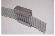
Slide the belt through both of the tension blocks so that the taps are both on top. Then place both wedges at the end of the belt.
