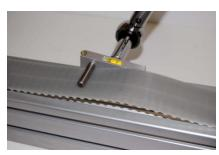
Move the tension block to the end of the actuator. Then place the tensioning tool at the middle of the belt.
