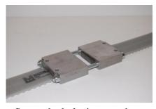
Screw the bolts in enough so that the bolts come out just a few threads past the nut.
