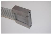
Pull the belt to tighten the wedge and the belt within the tension block.
