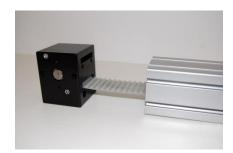
Insert the belt into the slot closest to the bottom. Push the belt in till it comes out the top.
