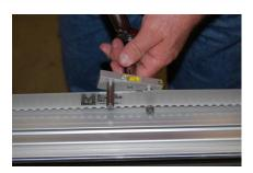
Move the tension block to the end of the actuator. Then place the tensioning tool at the middle of the belt.
