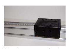
Move the cart over top the clamp and bolt in using the fixed holes. Be sure to have the fixed holes facing the drive side.
