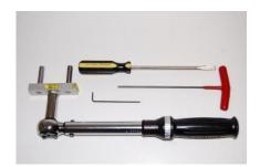
The tools you will need include a torque wrench (lb. in.), tensioning tool, M2 and M3 allen wrench, and a flathead screwdriver.
