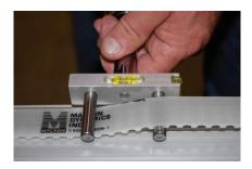
Set the wrench to the correct torque setting, adjust belt to achieve level position at the recommended torque.
