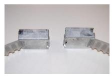
Pull the belt to tighten the wedge and the belt within the tension block.
