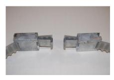
Place both wedges at the end of the belt so that the half-tooth is flush with the end of the wedge.
