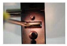
Using the screwdriver coax the belt upwards. Then push the belt till it stops at the top.
