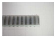
Using a *sharp* pair of tin snips, cut belt to length. Last tooth needs to be cut in half.
