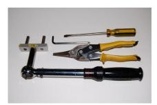
The tools you will need include a torque wrench (lb. in.), tensioning tool, tin snips, M5 allen wrench, and a flathead screwdriver.
