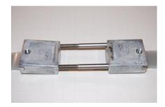
Place the bolts through the holes at the end of the tension block and into the other block. Be sure to put the heads of the bolts facing the drive side.
