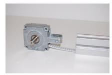
Insert the belt into the slot closest to the bottom.
