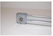
Push the belt in till it comes out the top. A screwdriver might be helpful to help along the pulley
