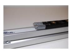
Attach the tension block to the cart using the shorter set of bolts on the drive side. The longer bolts will be used for the variable side.
