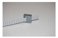
Slide the belt through both of the tension blocks so that the "M" is facing up.
