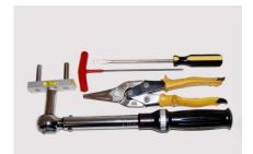
The tools you will need include a torque wrench (lb. in.), tensioning tool, tin snips, M3 allen wrench, and a flathead screwdriver.
