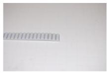
Using a *sharp* pair of tin snips, cut belt to length. Last tooth needs to be cut in half.
