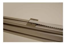
Place the belt clamp under the end of the belt so that the last tooth is in the first slot.
