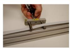
Move the cart to the end of the actuator. Then place the tensioning tool at the middle of the belt.
