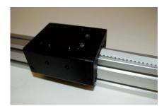
Move the cart over top the clamp and bolt in using the fixed holes. Be sure to have the fixed holes facing the drive side.
