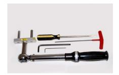
The tools you will need include a torque wrench (lb. in.), tensioning tool, M2 and a M3 allen wrench, and a flathead screwdriver.
