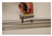
Set the wrench to the correct torque setting, adjust belt to achieve level position at the recommended torque.
