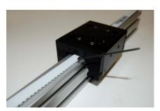
Tighten the set screws in the cart so that the belt becomes firm.
