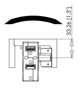
$M_x$  (static) = 575 in-lbs, 65 Nm.  $M_x$  (dynamic) = 327 in-lbs, 37 Nm.
