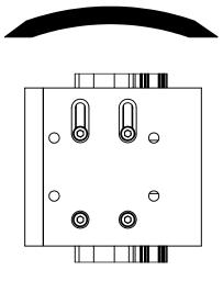
$M_z$  (static) = 309 in-lbs, 35 Nm.  $M_z$  (dynamic) = 177 in-lbs, 20 Nm.
