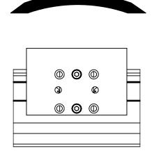
$M_y$  (static) = 309 in-lbs, 35 Nm.  $M_y$  (dynamic) = 177 in-lbs, 20 Nm.
