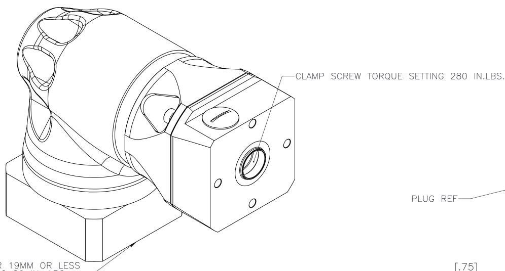
MOTOR INPUT SHAFT DIAMETER 19MM OR LESS CLAMP SCREW TORQUE SETTING 80 IN. LBS.
