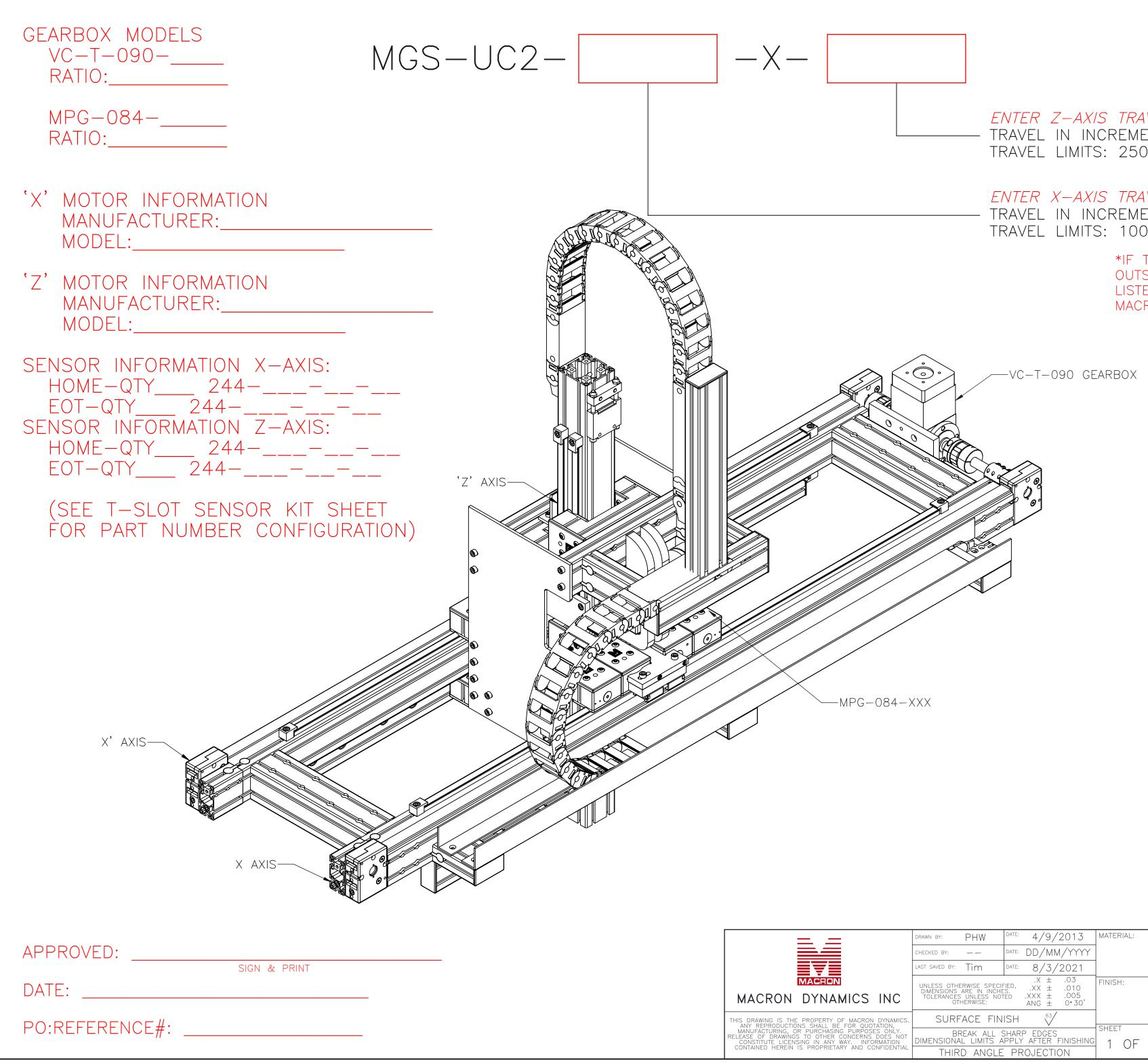
ENTER Z-AXIS TRAVEL - TRAVEL IN INCREMENTS OF 250mm TRAVEL LIMITS: 250mm-1000mm
