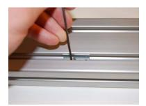
Then move the wrench forward to slide the T-Nut into place and into the slot.
