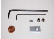
The tools and parts you will need include a M2 and a M4 wrench, a penny, an M3x10 bolt, the M8x8 and M8x6 set screws, and a sensor T-Nut.
