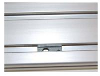
First place the T-Nut in the slot with the bigger of the two holes facing the driving pulley.
