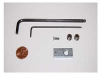
The tools and parts you will need include a M2 and a M4 wrench, a penny, an M3x10 bolt, the M8x8 and M8x6 set screws, and a sensor T-Nut.
