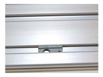
First place the T-Nut in the slot with the bigger of the two holes facing the driving pulley.
