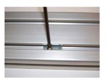
Use the M4 wrench to insert the appropriate set screw into the appropriate hole.
