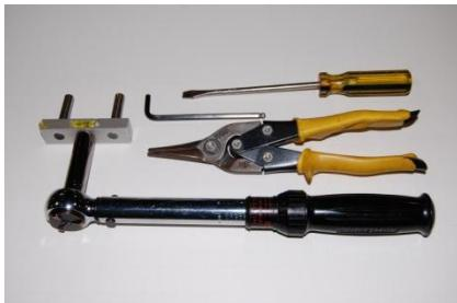
The tools you will need include a torque wrench (lb. in.), tensioning tool, tin snips, M6 allen wrench, and a flathead screwdriver.
