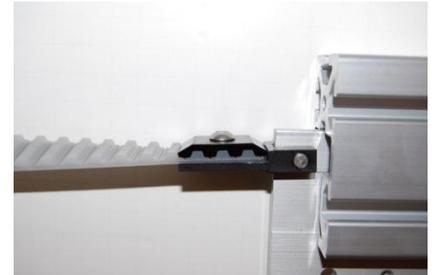
Bolt down the belt and clamp to the clevis. Repeat for other side of cart.
