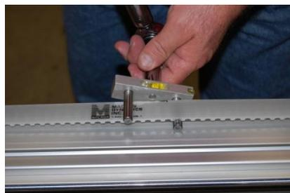
Move the cart to the end of the actuator. Then place the tensioning tool at the middle of the belt.
