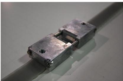
Screw the bolts in enough so that the bolts come out just a few threads past the nut.
