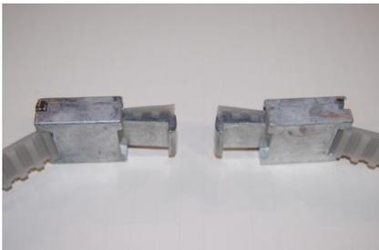
Place both wedges at the end of the belt so that the half-tooth is flush with the end of the wedge.
