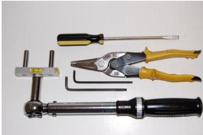
The tools you will need include a torque wrench (lb. in.), tensioning tool, tin snips, M5 and 5/32 allen wrench, and a flathead screwdriver.
