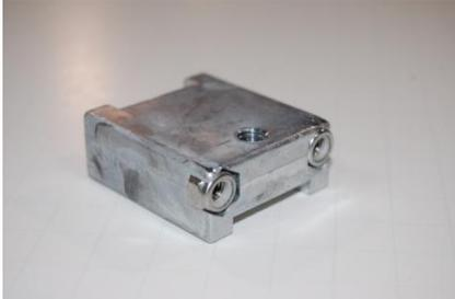
Insert nut in end of block. This may require use of a hammer.
