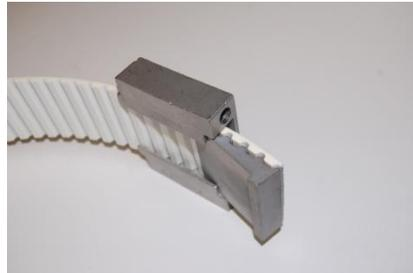
Place the wedge at the end of the belt so that the last tooth is flush with the end of the wedge.
