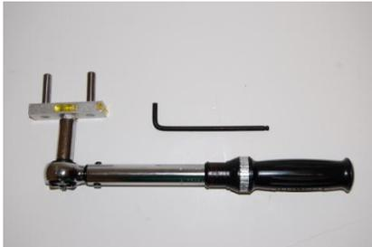
The tools you will need include a torque wrench (lb. in.), tensioning tool and a M6 allen wrench.
