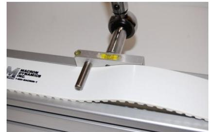
Set the wrench to the correct torque setting, adjust belt to achieve level position at the recommended torque.
