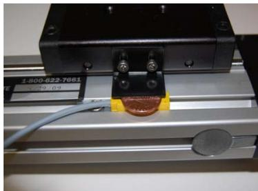
Then place a penny between the flag and sensor to be sure the flag is mounted at the correct distance from the sensor.
