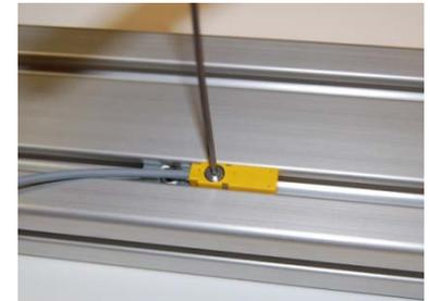
Place the sensor down with the wire running towards the drive shaft, and tighten with the M2 wrench.
